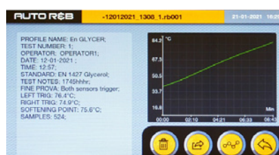
Saved test, complete with temperature/time graph
