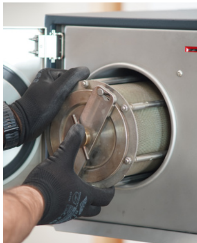
Placing the washing drum into the machine
