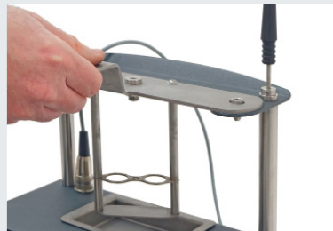
Detail of the PT100 probe holder drip tray for specimen holder, complete with handle
