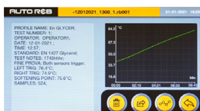
Saved test, complete with temperature/time graph
