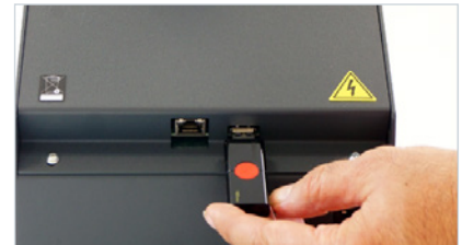
Communication ports are positioned on the rear side. LAN port is suitable for connecting to a PC or to LAN-hub, that creates a network with up to 32 independent units controlled by a single PC. USB port is used for data download to PC and firmware upgrade.
