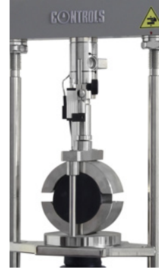
SPEEDLOADER EmS with Marshall accessories conforming to: EN 12697-34; ASTM D1559; ASTM D5581; ASTM 6927; AASHTO T245; BS 598-107; NF P98-0251-2; DIN 1996; CNR 30
