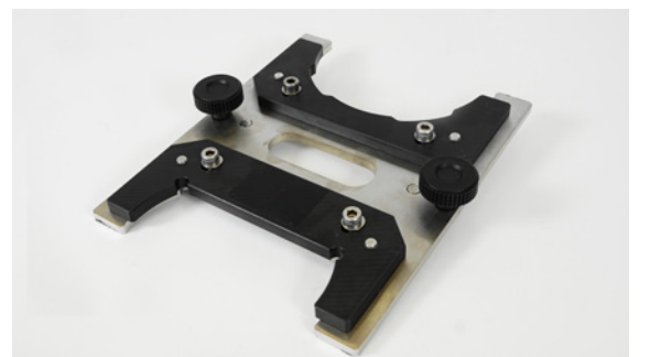
Overlay Test specimen jig
