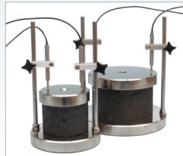
Permanent Deformation Test Set-up
