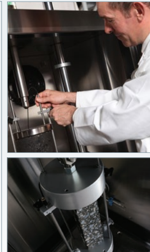
TSRST Thermal Stress Restrained Specimen Test
