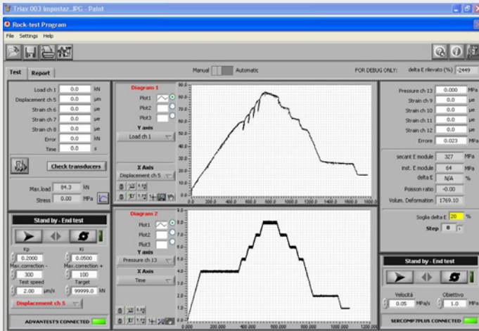
Screenshot of a stress-path triaxial test on rock performed with the ADVANCED system (load vs displacement and cell pressure vs time diagrams)
