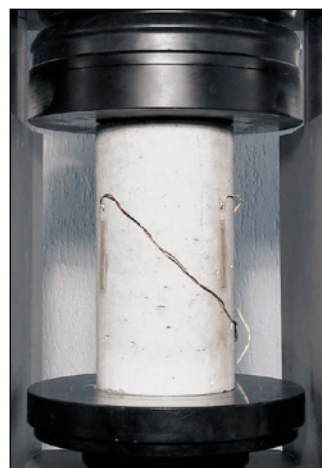
Specimen fitted with 55-C0222/F compressometers
