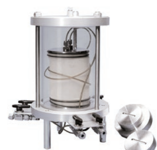
Permeability cell for contaminated soil
