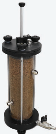
Constant Head permeability cell
