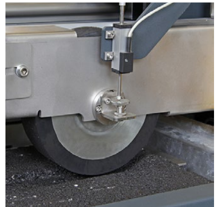
Detail of the motorized lifting system that raises the wheel assembly at the end of the test, making the use of hoists obsolete.
