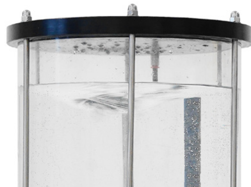
Initial water vortex during cavitation and vacuum application
