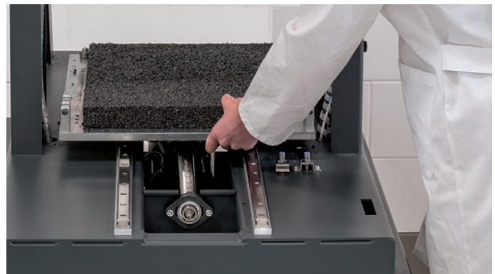
500 x 400 mm slab and lead-rolled ball screw system
