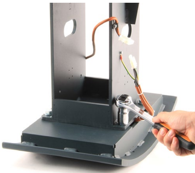
Detail of interchangeable sector head The sector head can be easily removed and replaced to produce slabs of the alternative dimensions.
