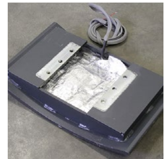
Heating system incorporated in mould base support
